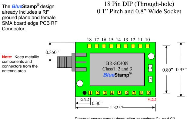
External power supply decoupling capacitors C1 and C2 are optional. C1 = 10uf Capacitor, 0805 Ceramic C2 = 0.1uf Capacitor, 0603 Ceramic
